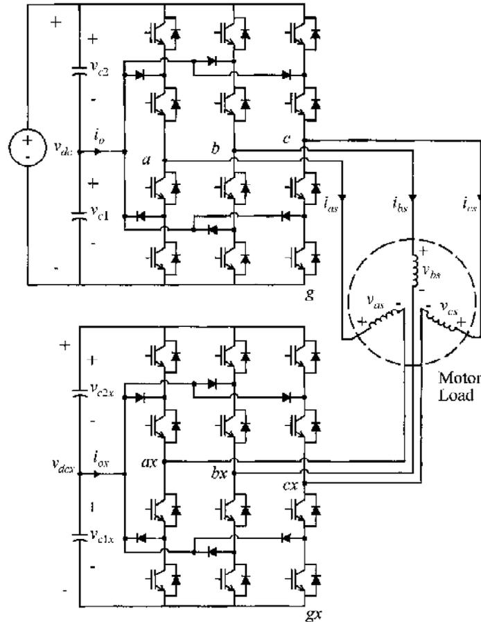
Fig. 4 . Cascade-3/3 multilevel inverter.
