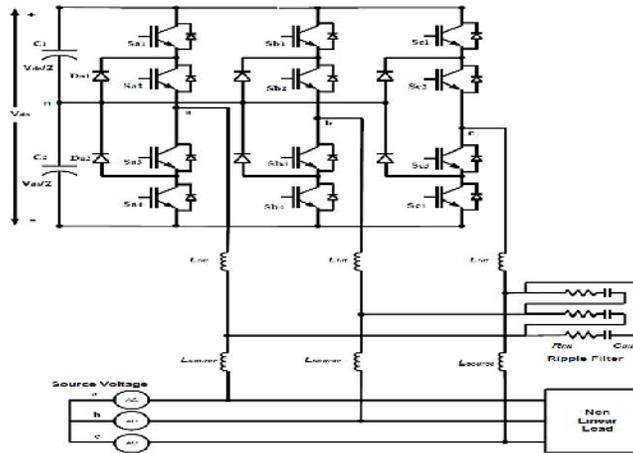
**Fig. 2.** Two and three-level VSI Block.
