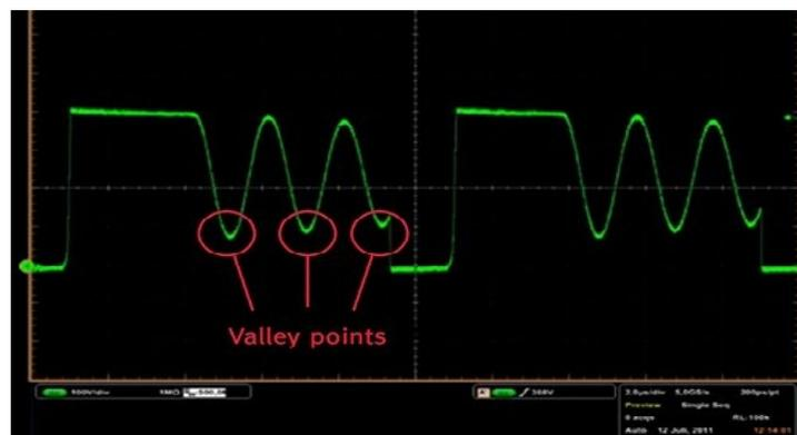
**Fig. 6.** Quasi-resonant switching waveform for a fly back converter (Courtesy of Infineon Technologies).
