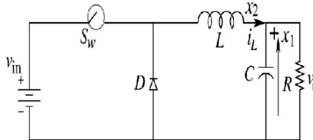
Fig. 2. Dc-dc buck converter topology.
