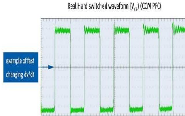
**Fig. 5.** Manufacturers increase  $dv/dt$  to minimize overlap and improve efficiency (Courtesy of Infineon Technologies).
