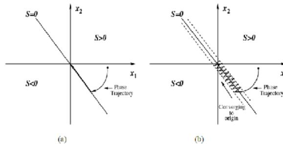
**Fig.1.** Phase Plot for (a) ideal SM Control (b) actual SM control.
