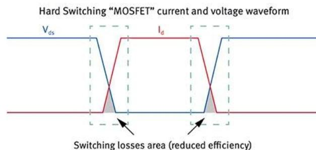
**Fig. 4.** Voltage regulator losses occur during voltage/current overlap when the MOSFET switches (Courtesy of Infineon Technologies).
