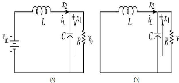
Fig. 3. Buck converter circuit when switch: (a) turns on (b) turns. Off.
