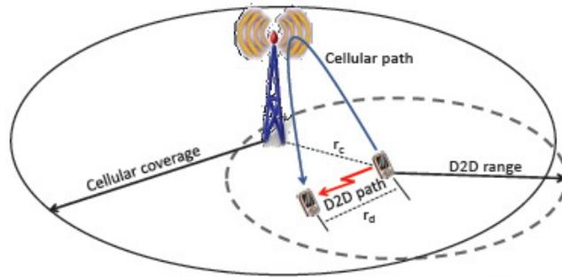
**Fig. 3.** Device-to-device (D2D) communication.
