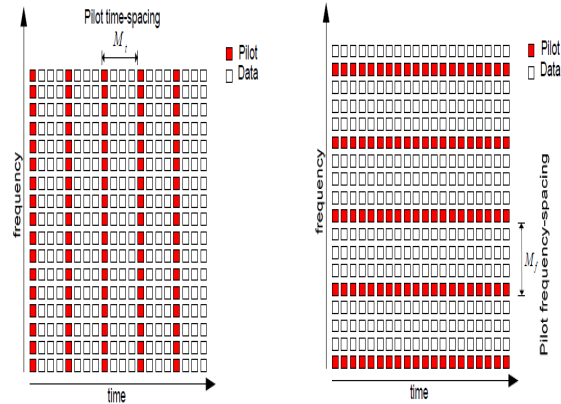
(a) All frequency-time spaced pilot allocation (b) Frequency spaced - all time pilot allocation.
