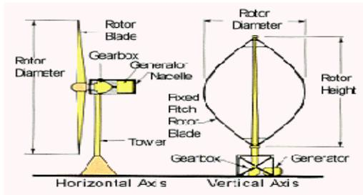
**Fig. 8.** Wind Turbine Configuration.
