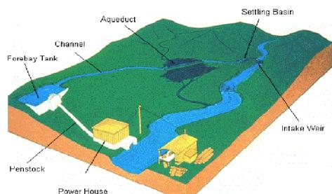
**Fig. 10.** Hydro Power Plant.
