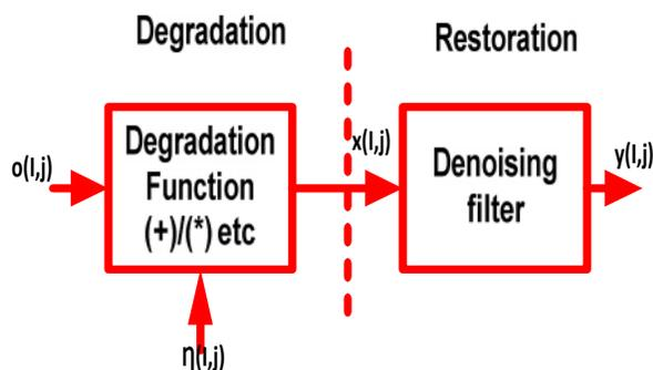
**Fig. 1.** Image degradation and restoration process due to noise only.
