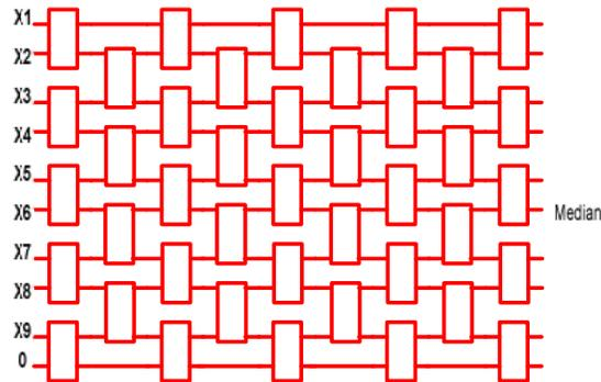
Fig. 5. Classical systolic array for shorting 9 pixel values using 41 nodes.
