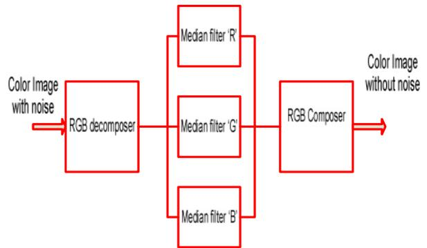
Fig. 4. Block diagram for image denoising.
