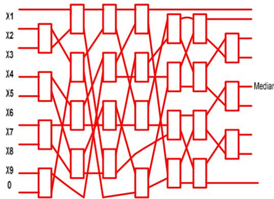
Fig. 6. Optimized systolic array for shorting 9 pixel values using 27 nodes.
