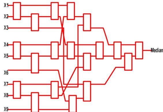
Fig. 7. Proposed systolic array for shorting 9 pixel values using 19 nodes.
