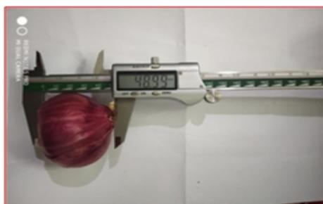
Fig. 1. Polar diameter ( $D_p$ ).
