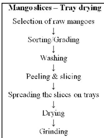
Fig. 3. Flow chart for Tray drying of mango slices.
