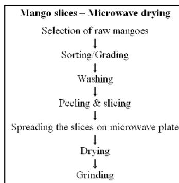
Fig. 5. Flow chart for microwave drying of mango slices.
