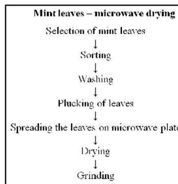
Fig. 6. Flow chart for microwave drying of mint leaves.
