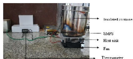
Fig. 7. Thermoelectric cooling system.
