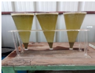
Fig. 2. Collection of wet biofloc using Imhoff cone.
