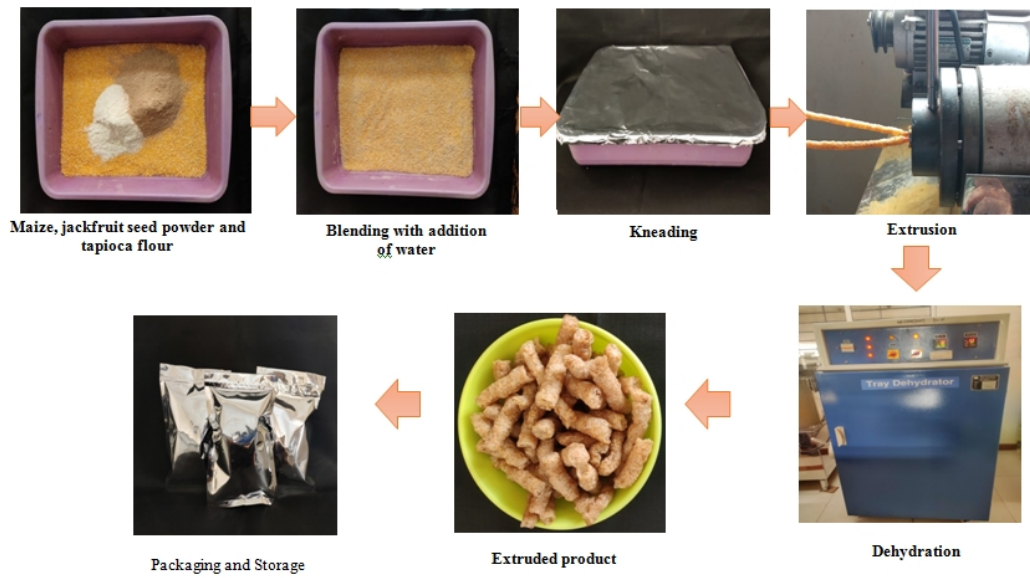
Plate 1. Flow chart for the preparation of jackfruit seed powder extruded product.
