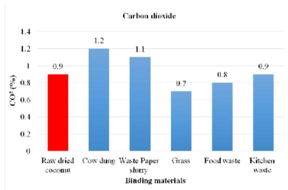
**Fig. 5.** Emission of carbon dioxide of tender coconut char with different binding materials.
