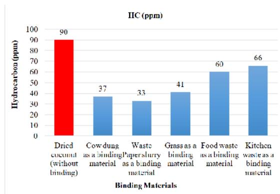
**Fig. 6.** Emission of hydrocarbon of tender coconut char with different binding materials.
