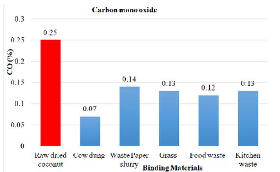
**Fig. 4.** Emission of carbon mono oxide of tender coconut char with different binding materials.
