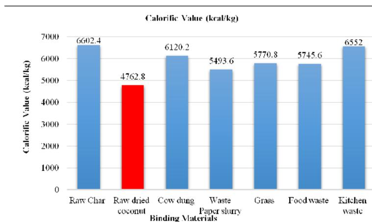
Fig. 3. Calorific value of raw dried tender coconut and its char with different binders.
