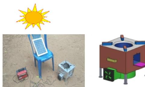
**Fig. 1.** Photograph of solar powered forced draft cook stove.
