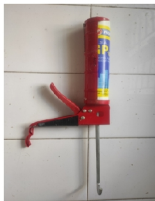
Fig. 2. Gun with silicon sealant.
