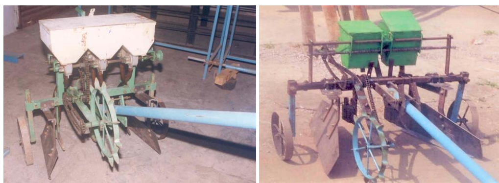
Fig. 1 a. Animal drawn broad bed former with seed cum ferti-drill; b. Broad bed former cum inclined plate planter.
