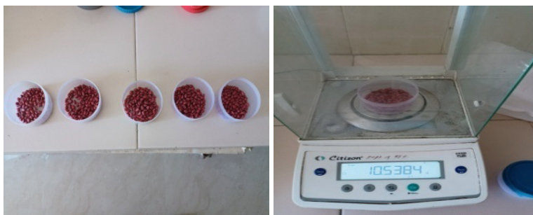
Fig. 7. Measurement of hundred seed weight of cotton seeds.
