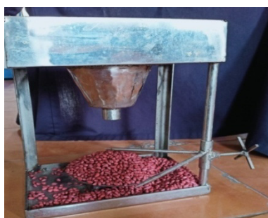
Fig. 8. Measurement of angle of repose of cotton seeds.
