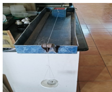
Fig. 9. Measurement of coefficient of friction of cotton seeds.
