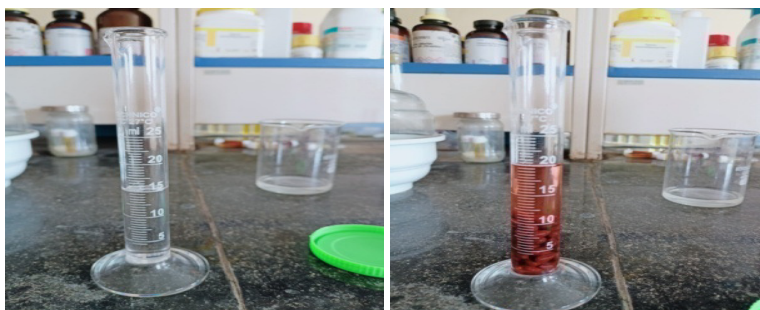
Fig. 6. Measurement of true density by toluene displacement.
