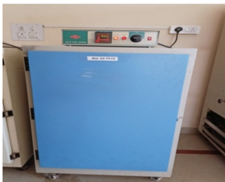
Fig. 4. Measurement of moisture content of cotton seeds using hot air oven.
