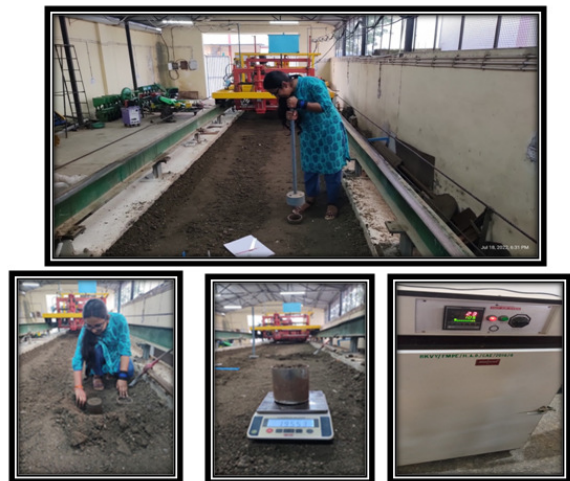
Plate 2: Procedure for measuring bulk density of the soil for the experiment.
