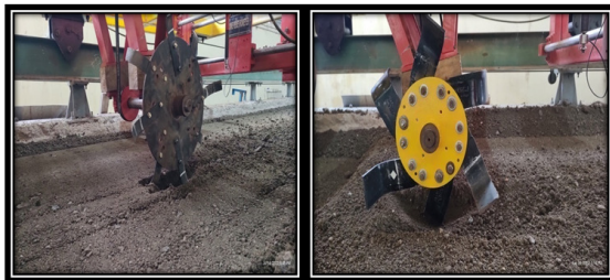
Plate 1. L and J-shaped rotary blade during test under soil bin
