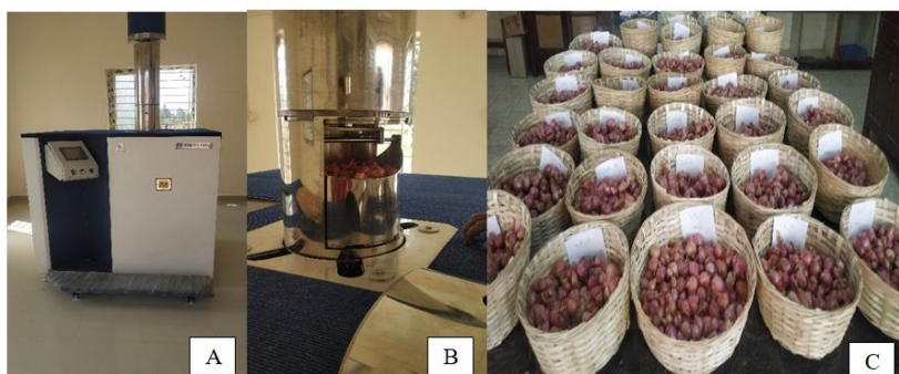
Fig. 1. A) Gamma irradiation chamber B) Irradiation treatment for onion bulbs C) storage of onion bulbs after treatments at ambient storage conditions.
