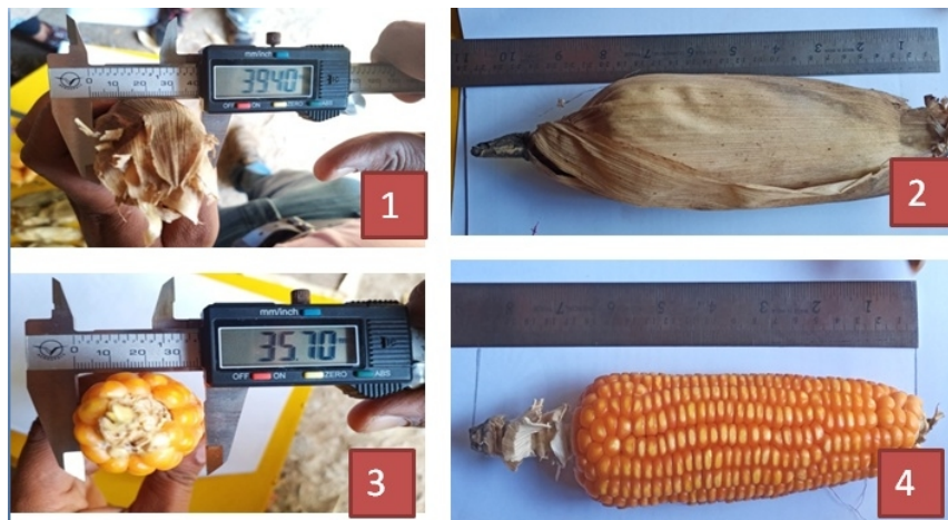
Fig. 1. Measurement of the dimensions of whole (1 and 2) and dehusked maize cob (3 and 4).
