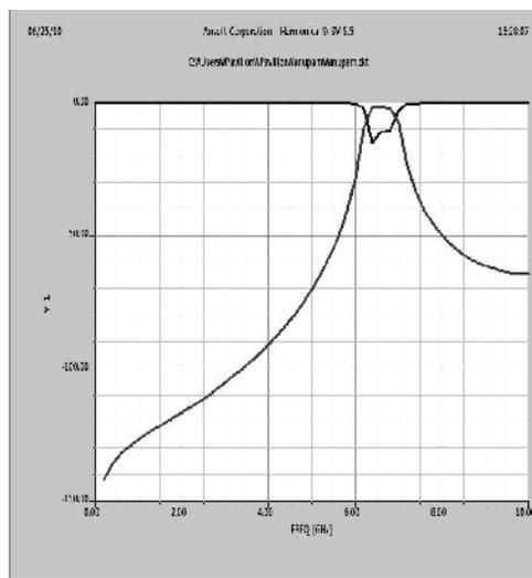
Fig. 6. Simulated response of the parallel-coupled line band pass filter.
