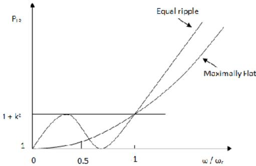
**Fig. 3.** Maximally Flat response and equal ripple response for a low pass filter for a finite order filter.
