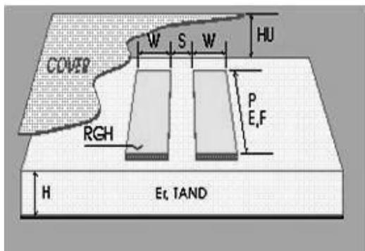
Fig. 4. A prototype for N=1 parallel-coupled line bandpass filter.
