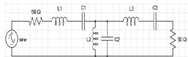
Fig. 1. Lumped circuit representation of a Bandpass filter.
