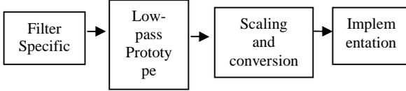
**Fig. 2.** Flow of steps required for design using insertion loss method.
