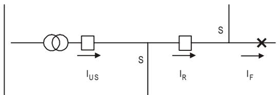
Fig.2. Typical feeder with addition of DG up line recloser.
