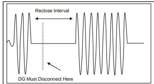
Fig.3. Fault current and Reclose interval.
