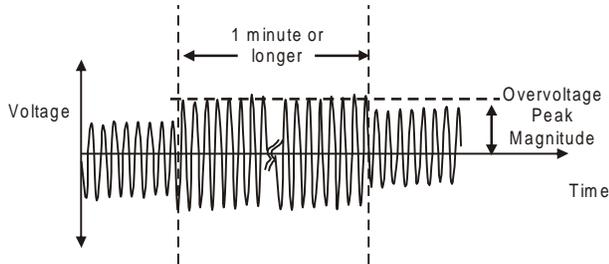
Fig.1. Typical overvoltage waveform [4].
