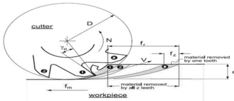
**Fig. 2** Basics of peripheral (slab) milling operation
