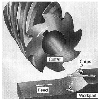
**Fig. 1.** Milling operation.
