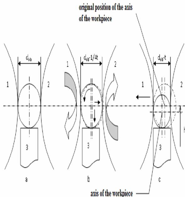
**Fig. 1.** Scheme of instant positioning of the work piece when in-feed grinding (a. starting the process; b. intermediate position of the work piece; c. position after one revolution of the work piece; 1. grinding wheel; 2. regulating wheel; 3. leading slide ).
