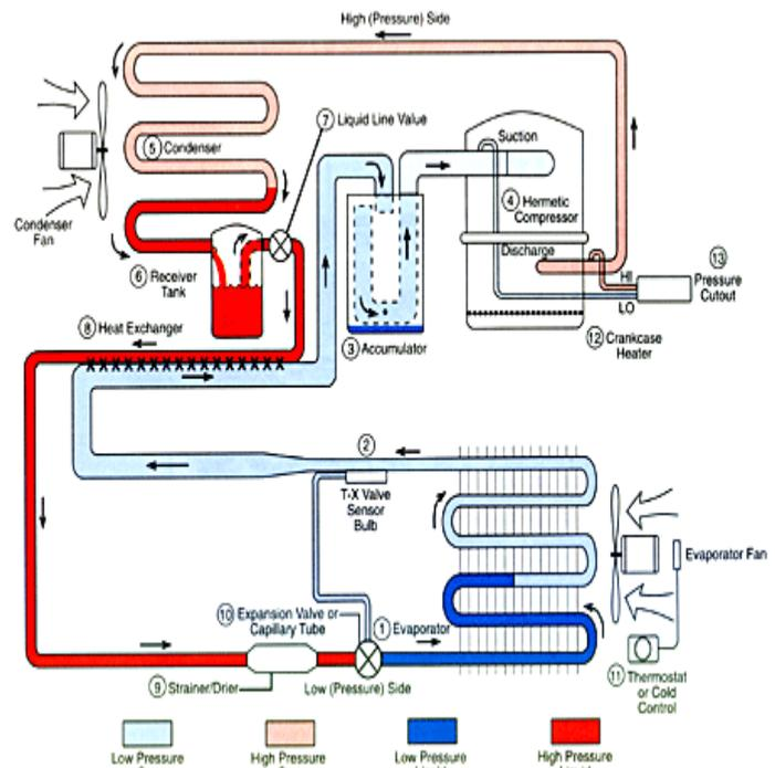
Fig. 2. Basic refrigeration cycle.
