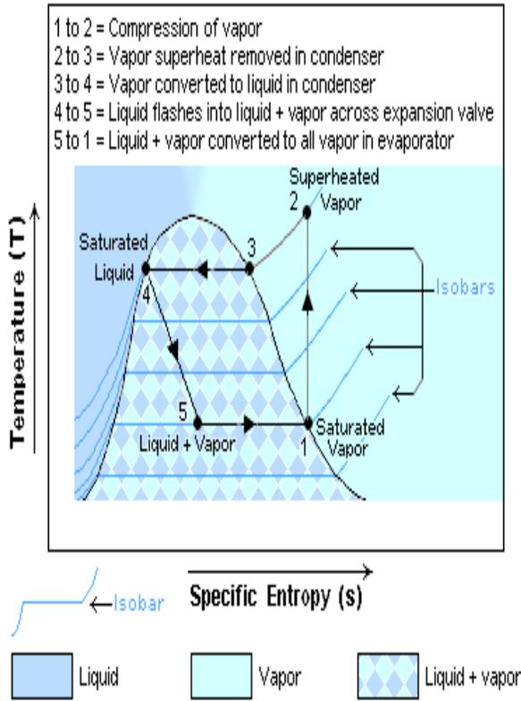
Fig. 5. Temperature-Entropy diagram.
