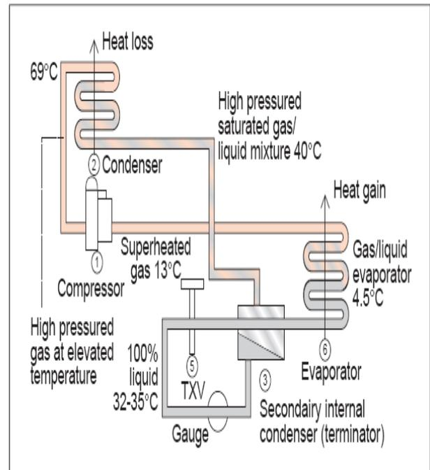
**Fig. 4.** Liquid line system diagram.
