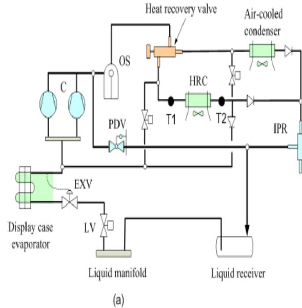
**Fig. 3.** Supermarket refrigeration system with heat recovery.
