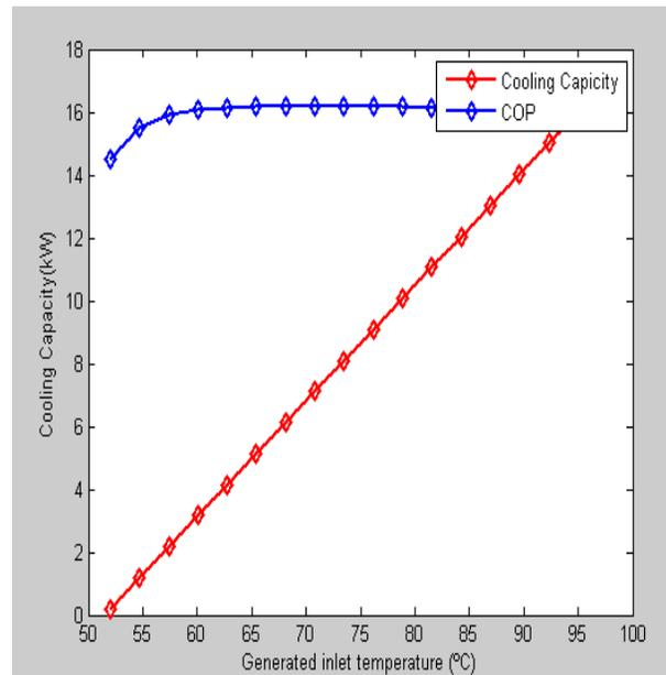
Fig. 6. Effect of generator inlet temperature on cooling capacity and COP.
