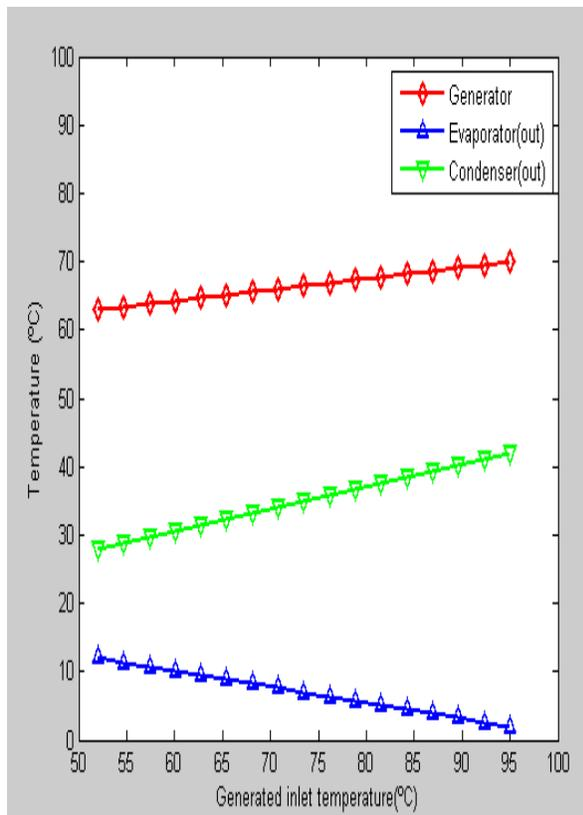
**Fig. 8.** Effect of generator inlet temperature on generator, evaporator and condenser temperatures.
