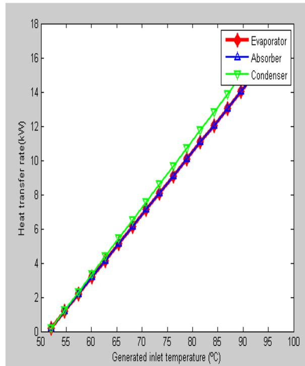
Fig. 7. Effect of generator inlet temperature on evaporator, absorber, condenser and generator heat transfer rates.
