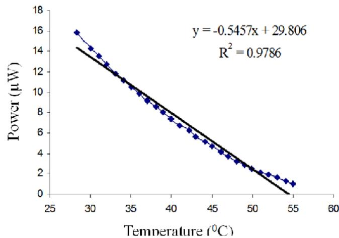
Fig. 4. Variation in power with temperature for second combination.
