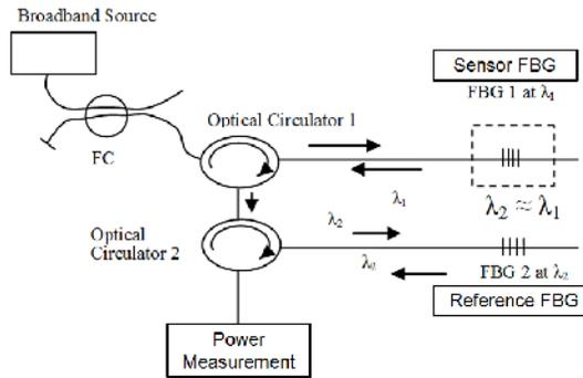
Fig. 1. Schematic of Setup for power measurement scheme.
