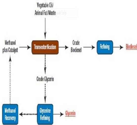
Fig. 2. Basic Process of Bio Diesel [13].
