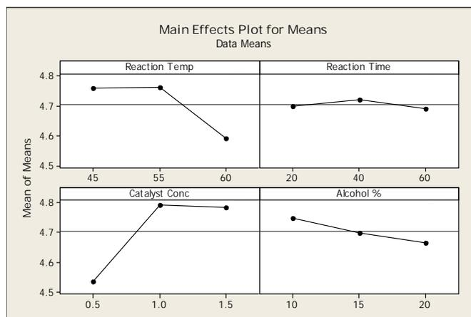
Fig. 7. Main Effects Plot for Means for Viscosity.
