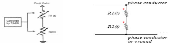
Fig. 3. HIF model using two time-varying resistances.
