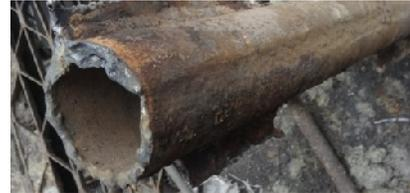
**Fig. 6.** Thickness Reduction due to fly ash Boiler-III SGP NFL Naya Nangal.
