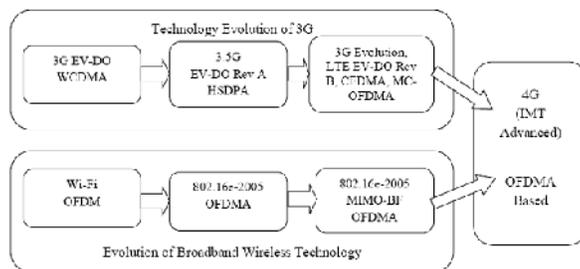
**Fig. 1.** Evolution Path of Mobile Technologies towards 4G WiMAX
