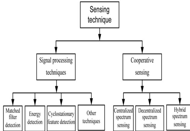
Fig. 1. Various Spectrum Sensing techniques.
