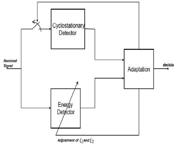
**Fig 3.** Hybrid Spectrum sensing Detector (HSD) architecture.
