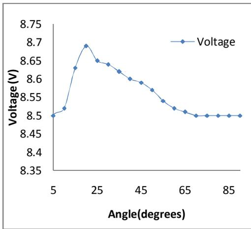
Fig. 6. Optimum trough angle for Single mirror concentrator.
