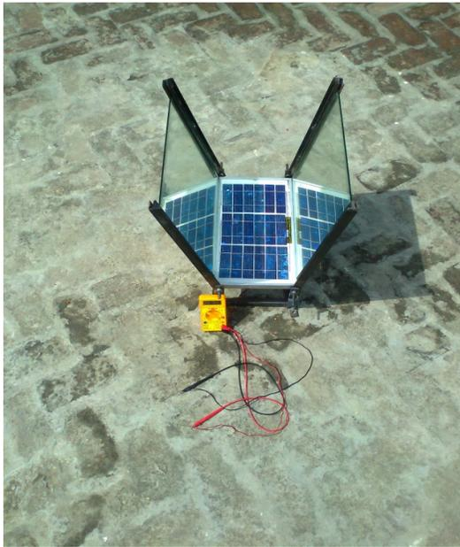
Fig. 1. PV-V-trough without cooling.
