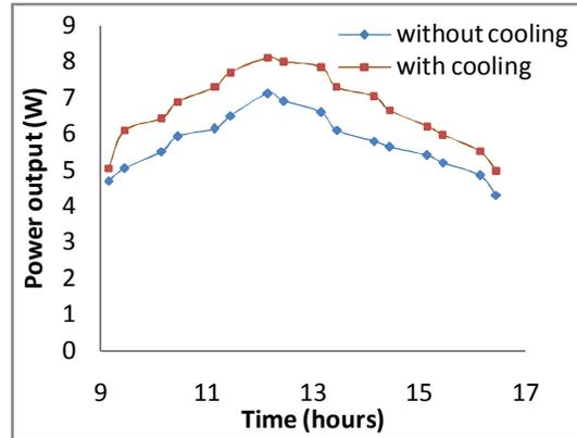
Fig. 2. Output comparison for Simple PV panel.
