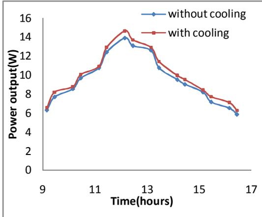
Fig. 5. Output comparison for PV-CPC.
