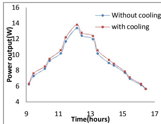
Fig. 4. Output comparison for PV-V-trough concentrator.
