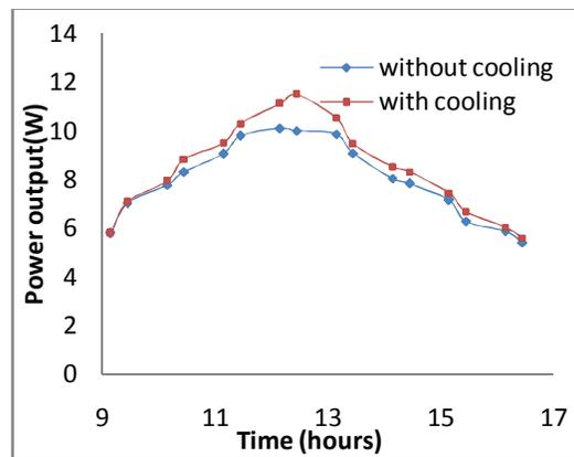
Fig. 3. Output comparison for PV-single mirror concentrator.
