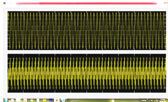
Fig. 5. Simulation result of grid injected voltage and current.
