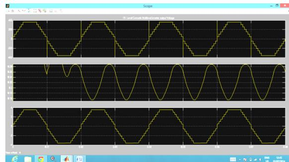
Fig. 4. Simulation result 15 level inverter for PV system.
