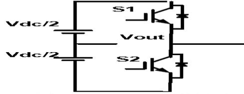
Fig. 2. One phase of a cascaded Half bridge multilevel inverter.
