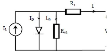
$$I_A = N_p [I_L - I_0 \{ \exp [q/kT_c (V_A / N_s) + (I_A R_s / N_p)] - 1 \} - (N_p / R_p) [(V_A / N_s) + (I_A R_s / N_p)]]$$
