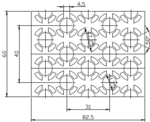
(b) Top view of interrupted half annular groove fin.
