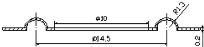
**Fig. 1.** Geometric model of heat exchanger with interrupted half annular groove fin.
