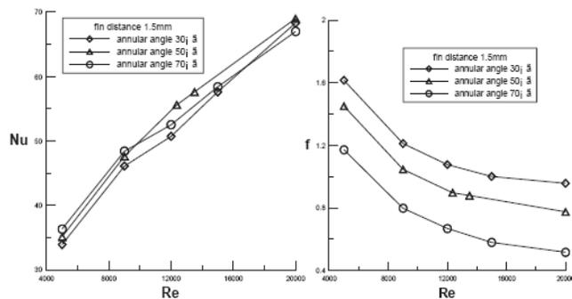
**Fig. 11.** Heat Transfer Performance and Pressure Drop Factor Curves for Interrupted Annular Groove Fin Unit with Attack Angle = 30,50,70.
