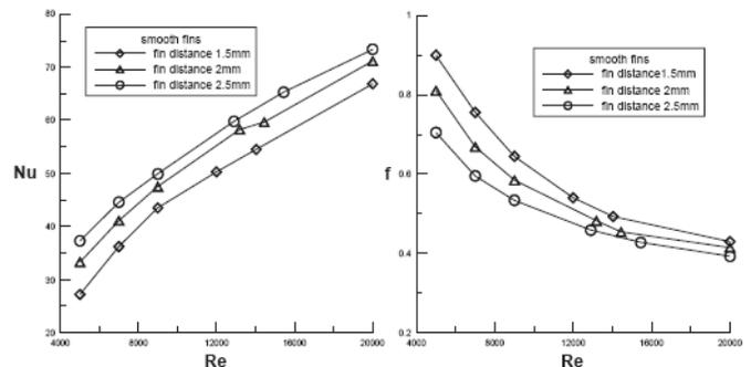
Fig. 7. Heat Transfer and Pressure Drop Factor Curves for Smooth Fin Unit with Fin Spacing = 1.5mm, 2mm, 2.5mm.
