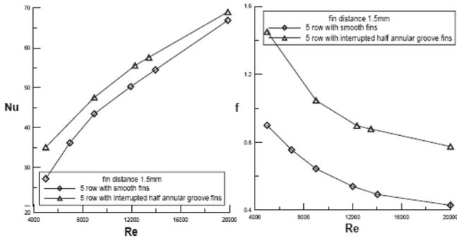
**Fig. 9.** Comparison of Heat Transfer and Pressure Drop between Smooth Fin Unit and Interrupted Annular Groove Fin Unit (Fin Spacing = 1.5mm).
