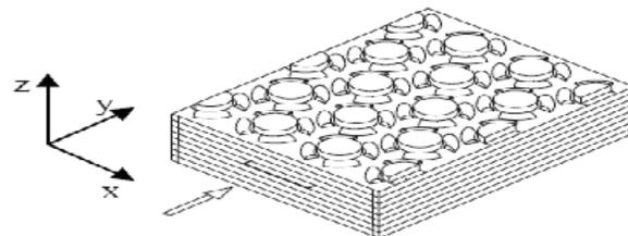
(a) Sketch of heat exchanger with interrupted half annular groove fin.
