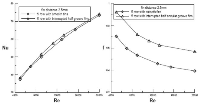
**Fig. 10.** Comparison of Heat Transfer and Pressure Drop between Smooth Fin Unit and Interrupted Annular Groove Fin Unit (Fin Spacing = 2.5mm).
