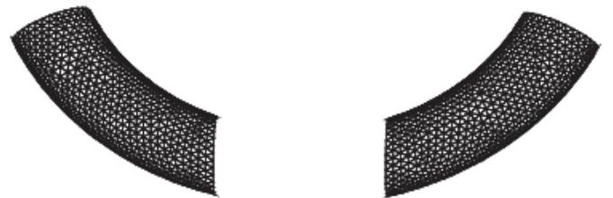
(b) Mesh of Annular groove Fig. 3 Calculation region and mesh. The proper number of mesh cells is verified with the criteria of cell number independence to Nu number and pressure drop coefficient.
