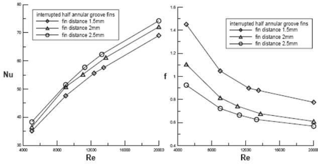
**Fig. 8.** Heat Transfer and Pressure Drop Factor Curves for Interrupted Annular Groove Fin Unit with Fin Spacing = 1.5mm.
