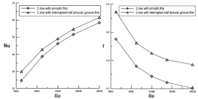
Fig. 6. Comparison of Heat Transfer and Pressure Drop between Smooth Fin Unit and Interrupted Annular Groove Fin Unit of Two Rows.
