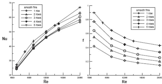
Fig. 4. Heat Transfer and Pressure Drop Curves of Smooth Fin unit with One to Five Rows.
