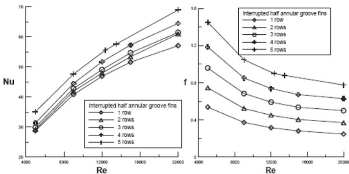
Fig. 5. Heat Transfer and Pressure Drop Curves of Interrupted Annular Groove Fin Unit with One to Five Rows.
