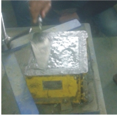
Fig. 7. Compaction of Concrete.
