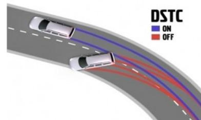
Fig. 1. Dynamic Stability and Traction Control.
