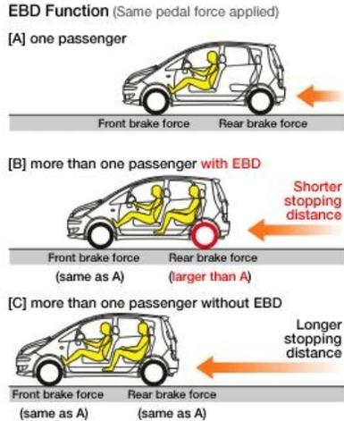
Fig. 2. Electronic Brake Distribution functioning.
