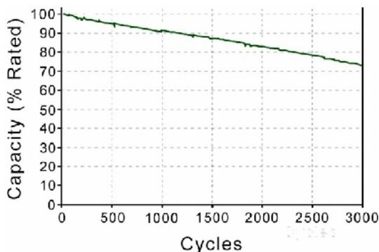
**Fig. 3.** Valence U27-36XP capacity retention.
