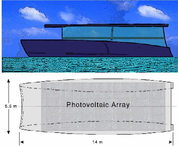
**Fig. 1.** Catamaran boat and available area for photovoltaic array.
