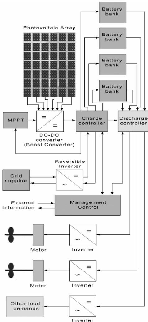
**Fig. 4.** Topology of solar-electric boat.
