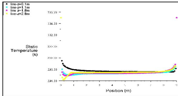
Fig. 7. Temperature profile at different heights for  $294^{\circ}K$  supply air temperature.
