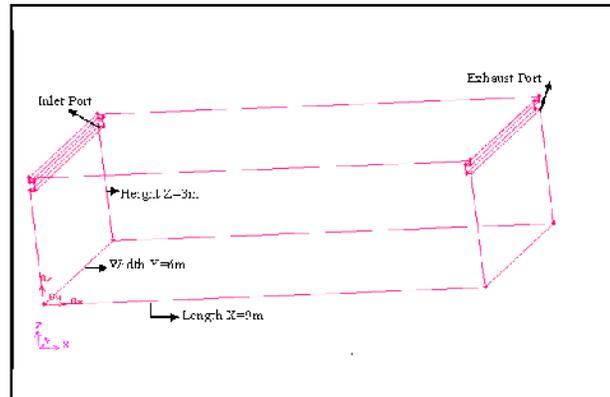
**Fig. 2.** The Geometrical model.
