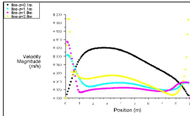
Fig. 10. Velocity profile at different heights for 0.2m/s at 298°K supply air temperature.
