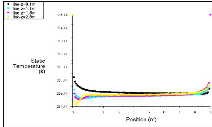
Fig. 9. Temperature profile at different heights for 298°K supply air temperature.
