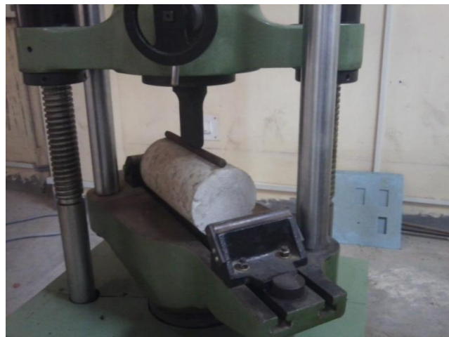
Fig. 1. Split Tensile strength test.
