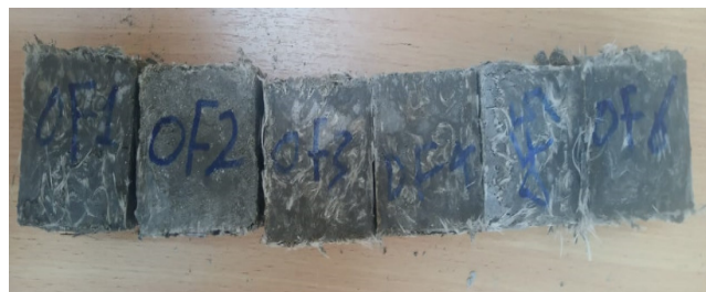
Fig. 5. Cubic's with Olive Oil Mill Wastewater and fibers.
