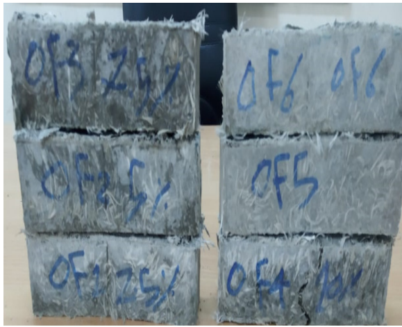
Fig. 9. The failure modes of the prisms with Olive oil mill wastewater and fibers.
