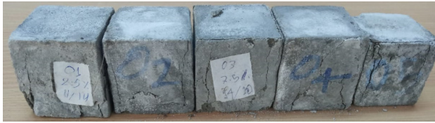
Fig. 6. Failure molds of the Cubic's with Olive Oil Mill Wastewater.
