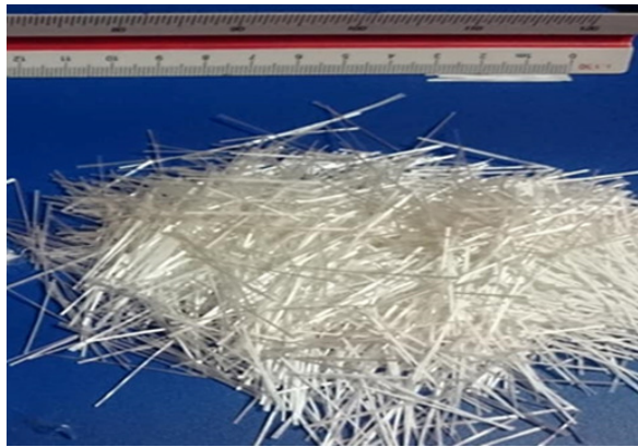
Fig. 1. AR glass fibers sample: 30mm length (A).
