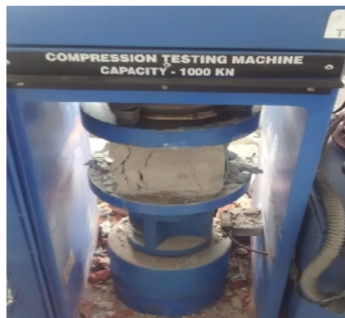
Fig. 1. Testing Cube Failure on Compression Testing Machine (CTM).
