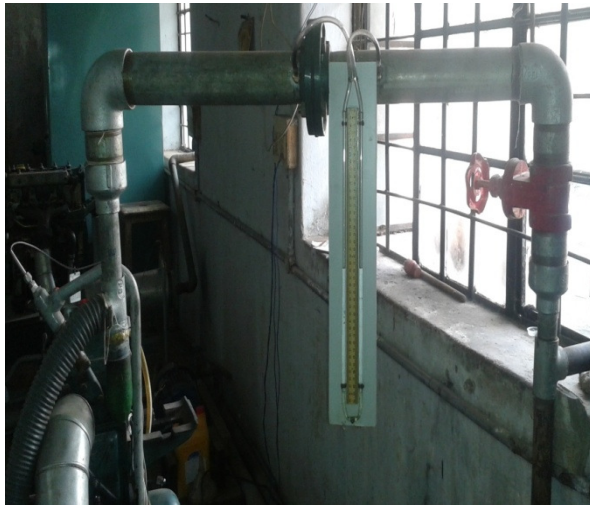
Fig. 1. Pictorial view of EGR arrangement to diesel engine.
