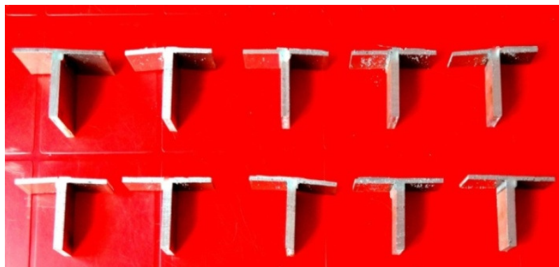
Fig. 5. Sample specimens produced by using the FSW method.
