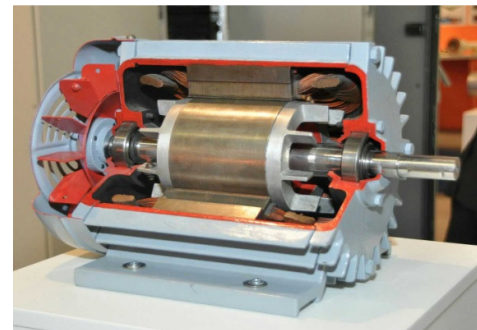
Fig. 12. Cut view of Electric Motor.
