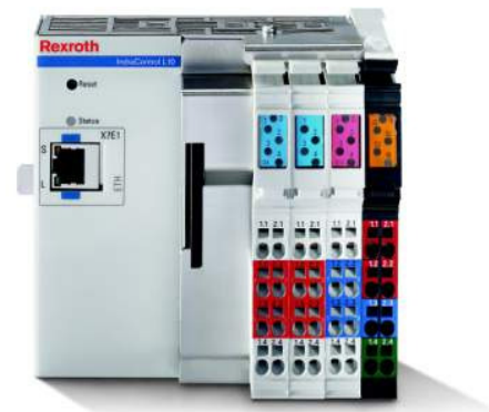
Fig. 2. Onboard input/output modules of PLC.
