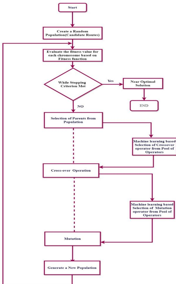
Fig. 3. Machine learning combine with Evolutionary algorithm.
