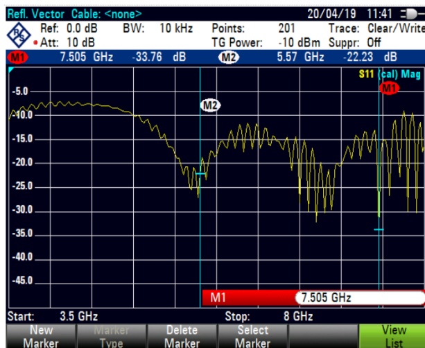
Fig. 16. Graph of VSWR for the optimally selected dimensions.
