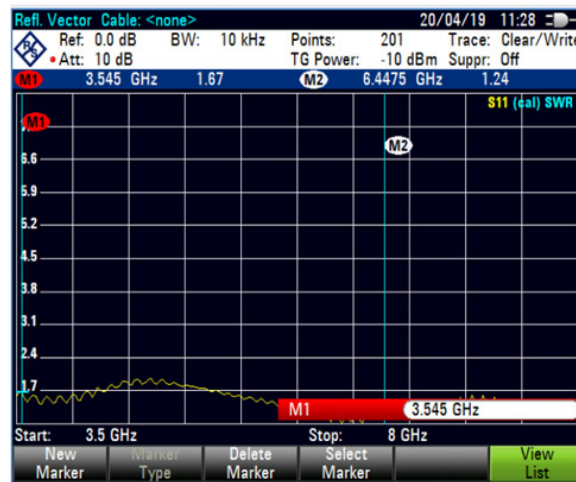
Fig. 15. Graph of s11 on VNA for the optimally selected dimensions.
