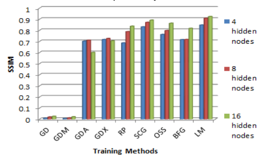
Fig. 8. Variation of SSIM values for GD, GDM, GDA, GD, BFG, RP, OSS, SCG, and LM training methods with hidden nodes of 4, 8 and 16 respectively.
