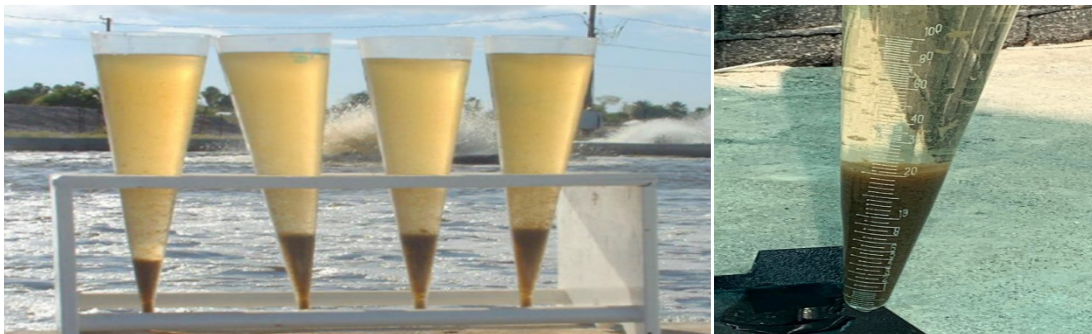
Fig. 5. Floc volume measurement with Imhoff cone.
