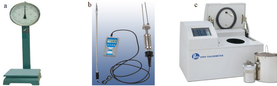
Fig. 1. Equipment used (a): Mechanical weighing scale 500kg (b): Universal moisture meter for biomass (c): Calorimeter 6100.
